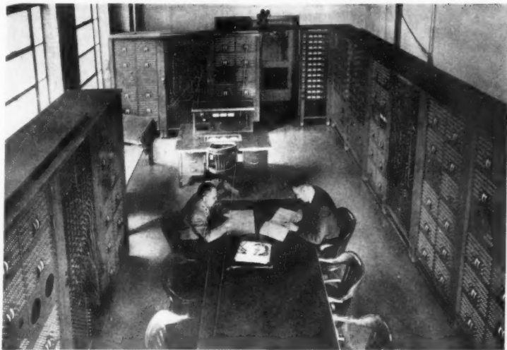
A-c network calculator allows setting up a power system in miniature and operating it with all combinations of loads and faults before any investment need be made.
